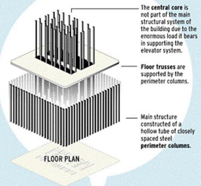
The central core is not part of the main structural system of the building due to the enormous load it bears in supporting the elevator system.
